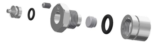
The Micro Port contains one septum held in a housing (the base) and kept in place by a hex nut. A pin screw axially positioned off-centre in the hex nut flange acts as a locking device once the hex nut is tightened to the right position.
